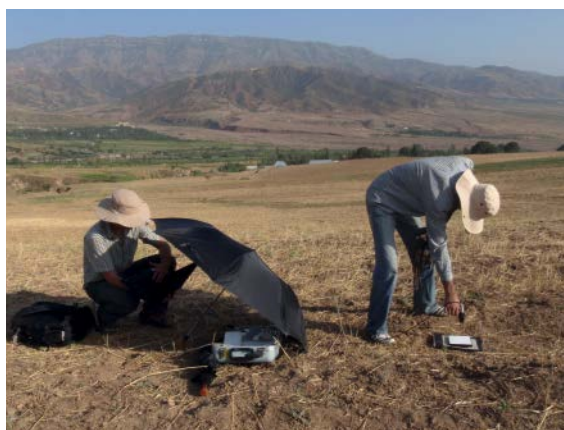
Soil spectral measurements in a field near Faizabad, Tajikistan. Photo: Bettina Wolfgramm, CDE
