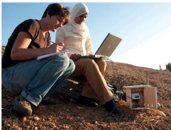
Measuring soil moisture using time domain reflectometers in Morocco. Photo: Hanspeter Liniger, CDE
