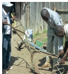
Photo 1: Demonstration of conservation tillage through shallow ripping of soil using draught animals. (Hanspeter Liniger) Photo 2 and 3: 'Victory' ploughs modified into ripper by replacing the plough blade by a metal tine to provide extra penetration. (Hanspeter Liniger and Frederick Kihara)
